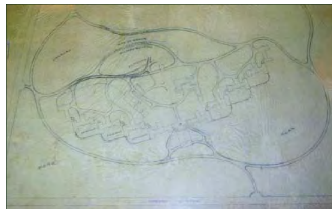
Figure III.6. “Plan of Grounds Belonging to the N.Y. State Insane Asylum, Buffalo, NY,” c. 1870. Note the angled alignment of the asylum building positioned over a ravine. Image Courtesy Buffalo Psychiatric Center. (R-BRO-FLO-1872-612-20)
