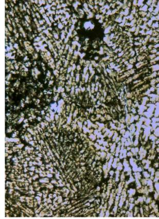
A particle of limestone, as compared to the lime mass shown in photo 9, 100x.
