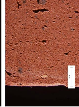
A cut corner of Sample 2 at 6X, showing less-frequent air voids near the edge of the brick. In this area, voids do not appear to be interconnected.
