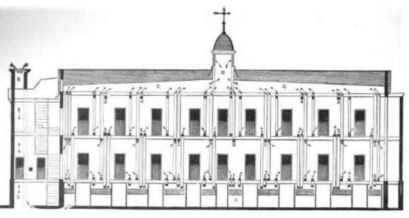
for the Buffalo asylum - unfortunately it was changed by the building contractor to internal downspouts in the built design, leading to eventual leaking, saturation and deterioration of the masonry.
