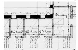
Fig A.19 Detail of a typical floor plan, Buffalo State Insane Asylum, showing shafts in the internal corridor wall for forced air circulation Image courtesy Houghton Library- Harvard University, H.H. Richardson Drawing Archives, Catalogue BLAA4
