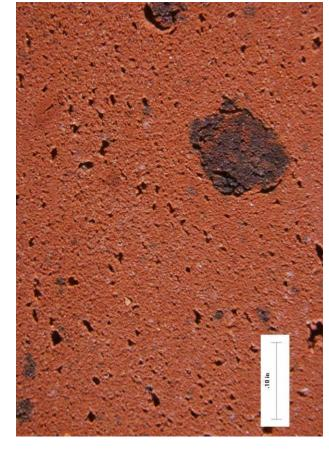
A cut corner of Sample 1 at 6X, showing small voids and a dense structure. Voids do not appear to be interconnected.
